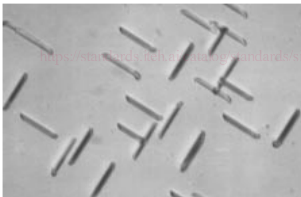
FIG. 17 Copper-3 Etch With Agitation, Oxidation Stacking Fault, 500x, p type, 10 ohm-cm, [100] (1100°C Steam, 80 minutes), 2 \mu m removal.
