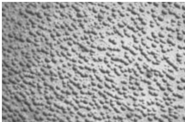
FIG. 18 Copper-3 Etch With Agitation, Shallow Pits (Haze), 500x, p type, 10 ohm-cm, [111], (1100°C Steam, 80 minutes), 2 \mu m removal
