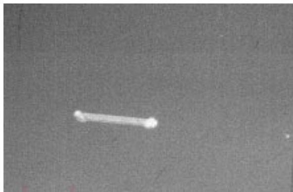
FIG. 1 Secco Etch With Agitation, Oxidation Stacking Fault, 1000x, [100], (1100°C Steam, 80 minutes), ~4 \mu m removal.
