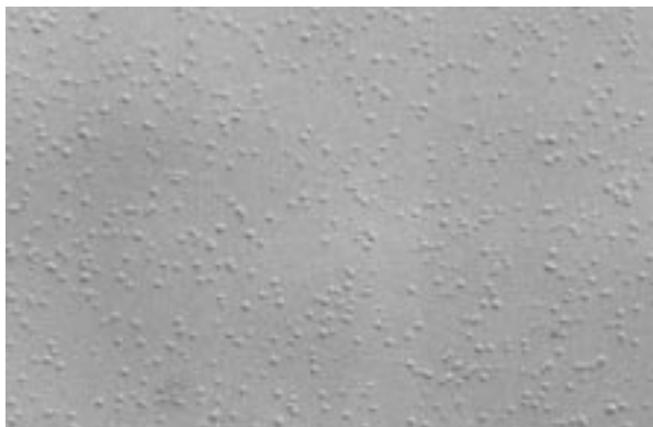
FIG. 15 Wright Etch With Agitation, Shallow Pits (Haze), 500x, Boron Doped [100], (1100°C Steam, 80 minutes).
