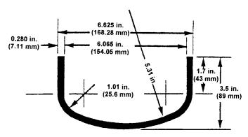
Note 1—Caps furnished to ANSI standards unless otherwise specified. Welding caps are formed from steel plate and are ellipsoidal in shape. The minor axis being equal to one half the major axis radii "R" and "r" closely approximate the actual semi-ellipsoidal shape. All dimensions in inches and are in accordance with ANSI B16.9.
