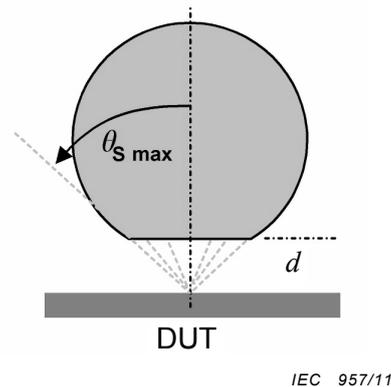
Figure 5b – Integrating sphere with large aperture
