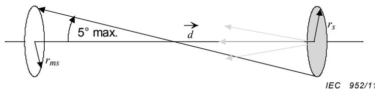
Figure 2 – Directional illumination with a flat source disk
