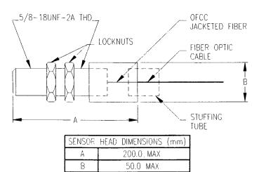
FIG. S4.1 Sensor Head Construction
