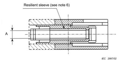
Figure 1a – Simplified receptacle housings interface
