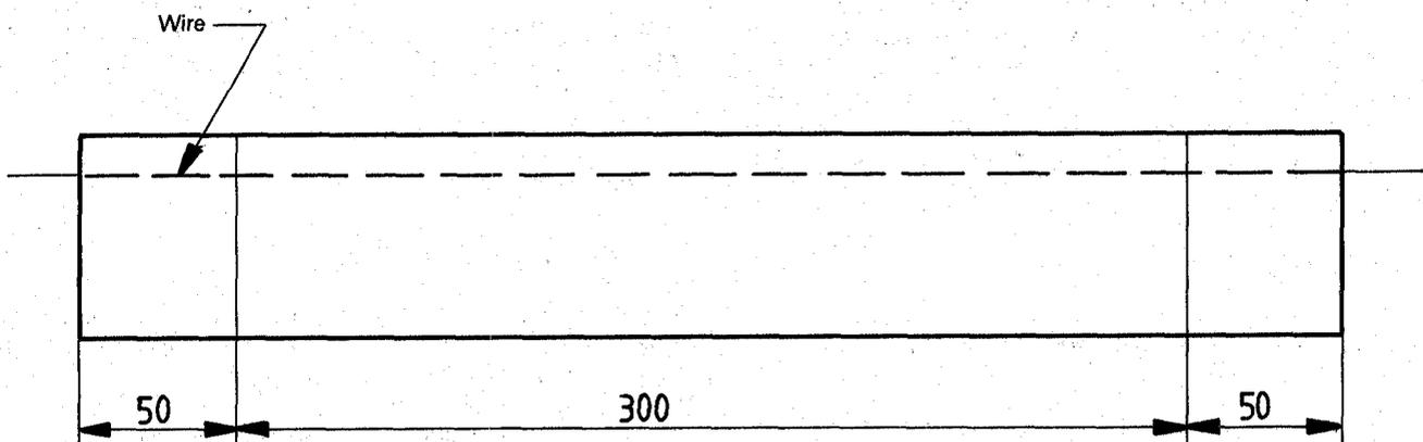
**Figure — Burning time test sample**
