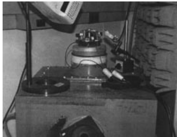
FIG. 1 Motor Mounted to Plenum Chamber
