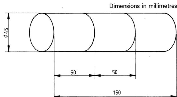
Figure 1 — Exposed protrusion test cylinder
