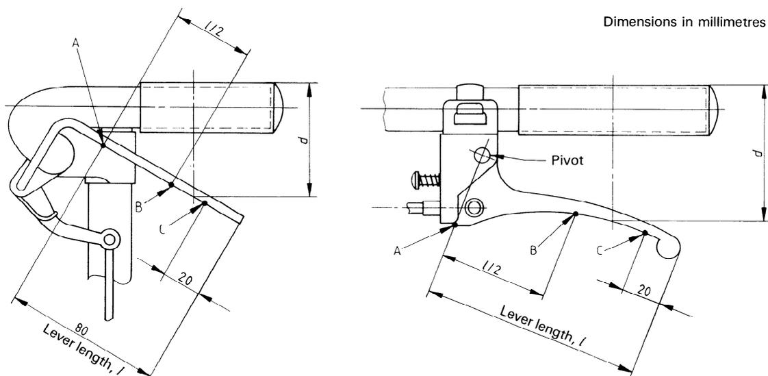
Figure 2 — Hand-brake lever dimensions
