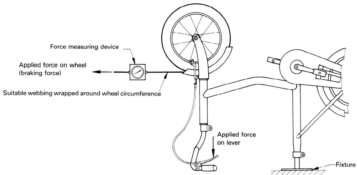
Figure 6 — Measurement of braking force from hand-brake
