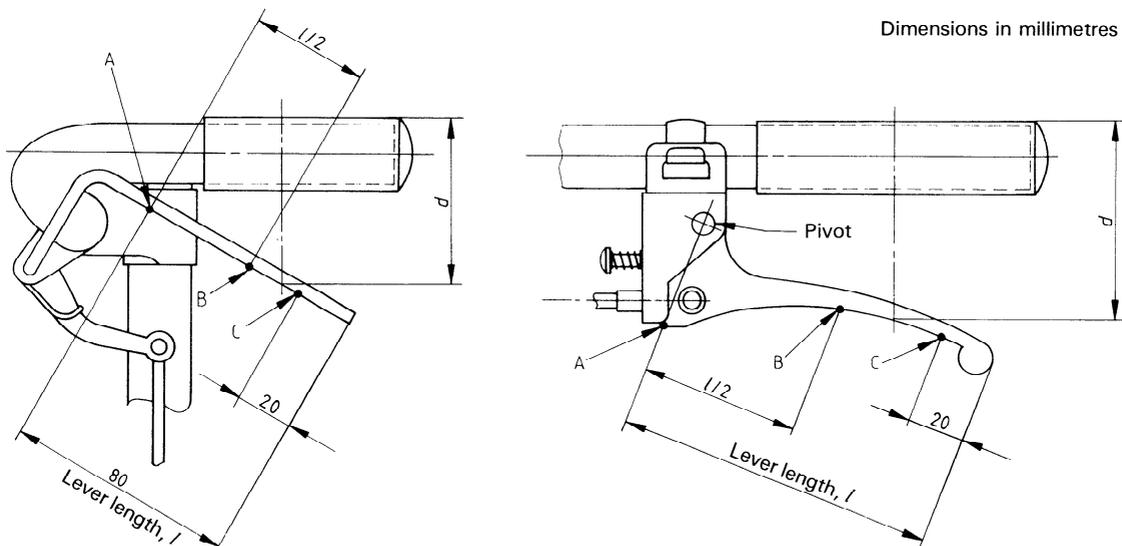
Figure 2 — Hand-brake lever dimensions
