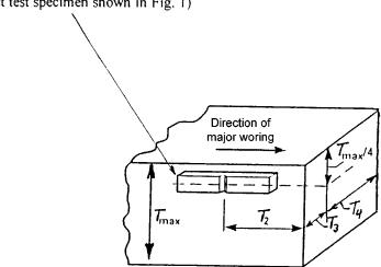
Note—For material with thickness T greater than 2 in. [50 mm],  $T_2=T_3=T_4 \ge T_{max}T_{max} = maximum$  heat treated thickness FIG. 1 Test Specimen Location for Quenched and Tempered Forgings
