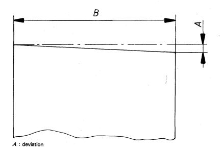
B: length or width of the sheet measured at right angles to an edge
