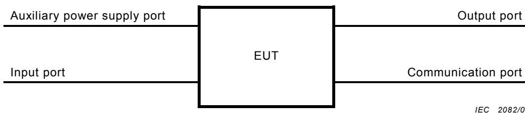
Figure 1 – Ports tested in this standard for measuring relays and protection equipment
