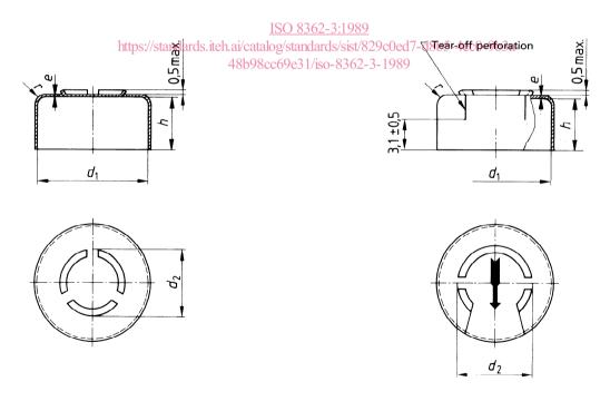
c) Type C – Aluminium cap with three-bridge tab
