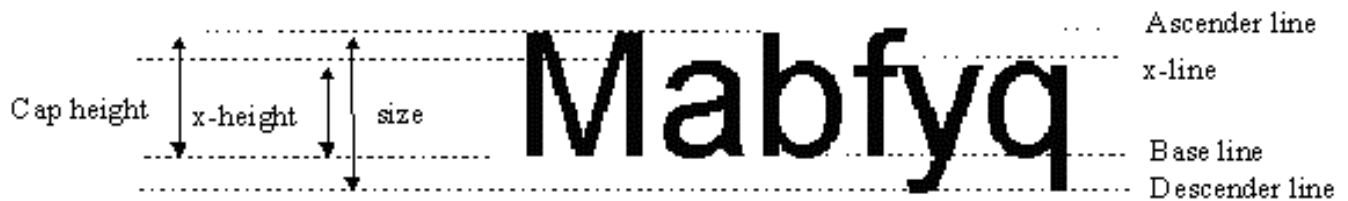
Figure 2 — Reference lines and dimensions
