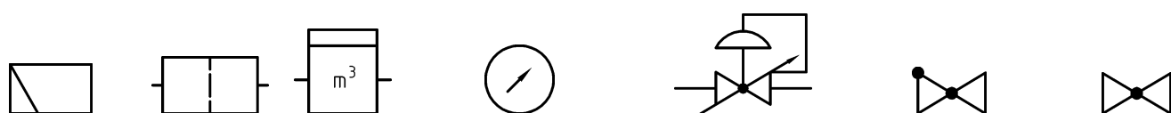
a) Control unit b) filter c) flow meter d) pressure gauge e) pressure reduction valve f) non return valve g) shot valve
