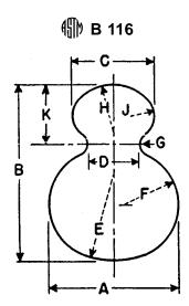
Note—For dimensions E, F and H the dimensional tolerance is ±0.016 in. (0.406 mm); for dimensions G and J the dimensional tolerance is ±0.008 in. (0.203 mm).
