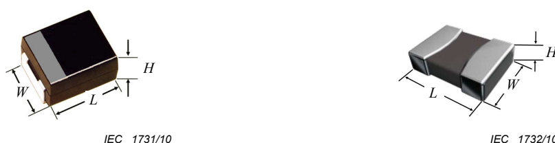
Figure 1a – Lead frame electrode terminal Figure 1b – Thin coating electrode terminal Figure 1 – Lead frame and thin coating types of surface mount capacitors and the specification of the dimensions ( L , W , and H )
