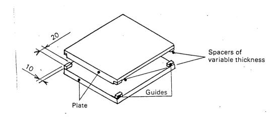
Figure 2 — Press mould type 2
