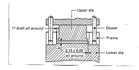
Figure 1 — Press mould type 1
