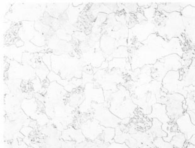
FIG. 1 Example of Replica Microstructure at 100\times LM. Material: See Specification A 335/A 335M, Grade P22. Etchant: 2 % Nital
