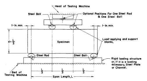
NOTE 1—This apparatus may be used inverted. If the testing machine applies a force through a spherically sealed head, the center pivot may be omitted, provided one load-applying block pivots on a rod and the other on a ball. NOTE 2-1 in, = 25.4 mm.
