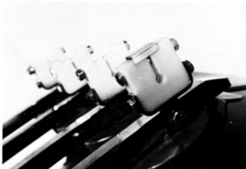
FIG. 6 Wear Block or Specimen Holder
