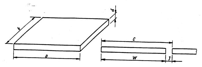
Co-ordinating size (C) = Work size (W) + Joint (J) Work size (W) = Dimension of the visible face (a) and (b)
