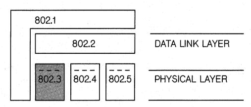
This family of standards deals with the Physical and Data Link Layers as defined by the ISO Open Systems Interconnection Basic Reference Model (ISO 7498 : 1984). The access standards define three types of medium access technologies and associated physical media, each appropriate for particular applications or system objectives. The standards defining these technologies are
