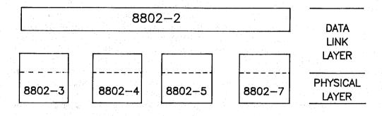
This family of standards deals with the physical and data link layers as defined by the ISO Open Systems Interconnection Basic Reference Model (ISO 7498 : 1984). The access standards define four types of medium access technologies and associated physical media, each appropriate for particular applications or system objectives. The standards defining these technologies are
