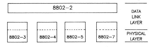
This family of standards deals with the physical and data link layers as defined by the ISO Open Systems Interconnection Reference Model (ISO 7498 : 1984). The access standards define four types of medium access technologies and associated physical media, each appropriate for particular applications or system objectives. The standards defining these technologies are
