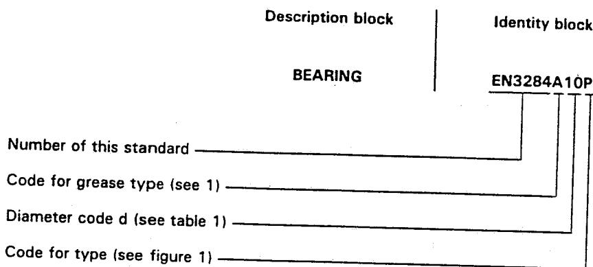
NOTE : If necessary, the code I9005 shall be placed between the description block and the identity block.
