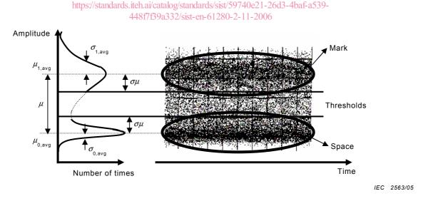
Figure 1 – Asynchronous eye-pattern and amplitude histogram
