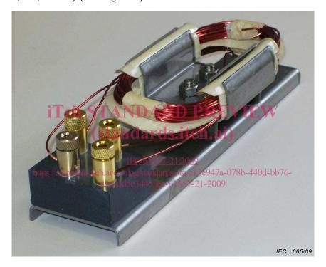
NOTE The additional height of the channel area in the GPM-TC allows for evaluation of three coils of winding wire and the extra pair of stand-offs allows for electrical testing of the additional coil.
