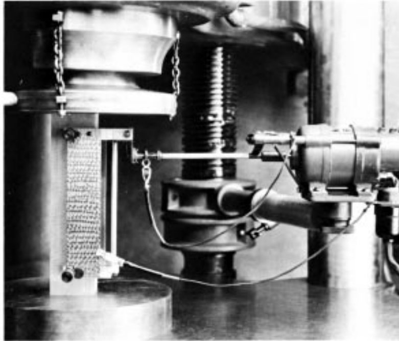
FIG. 8 Compression-Parallel-to-Grain Test Assembly Using an Automatic Type of Compressometer to Measure Deformations (The wire in the lower right-hand corner connects the compressometer with the recording unit.)
