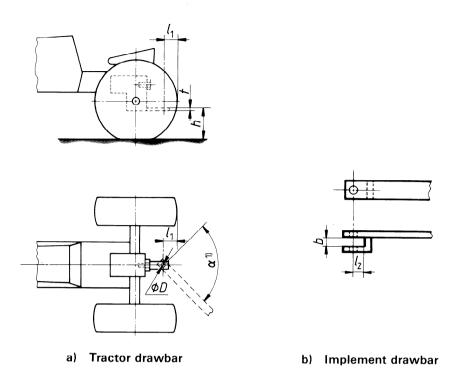
The tongue end of the tractor drawbar shall clear a clevis 51 mm wide mounted on an implement through a max. 90° swing to either right or left of the tractor drawbar centreline or implement tongue interference with the tractor tyre, whichever occurs first.
