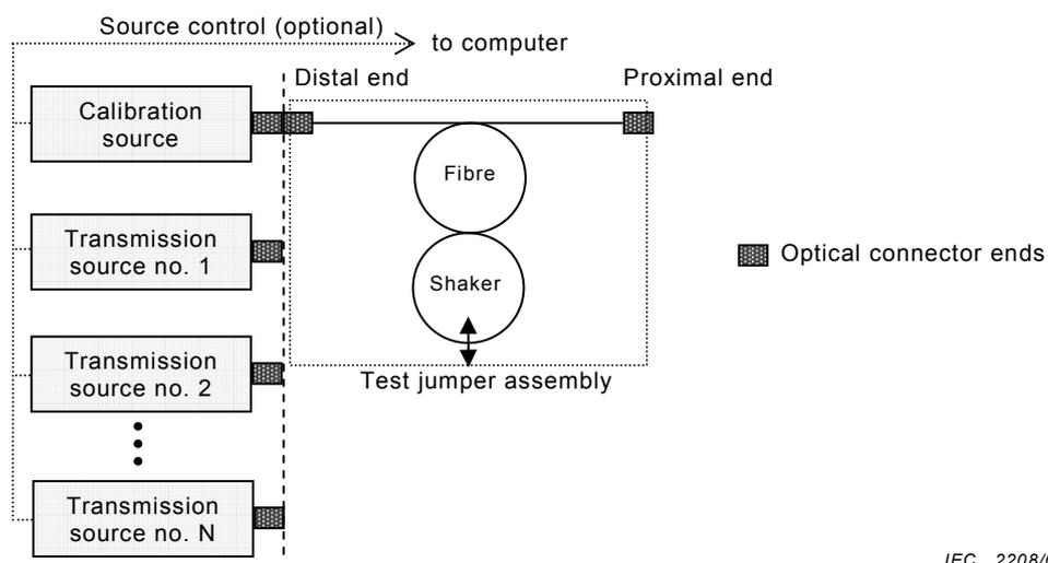
**Figure 2 – Typical set-up for transmission source measurement**
