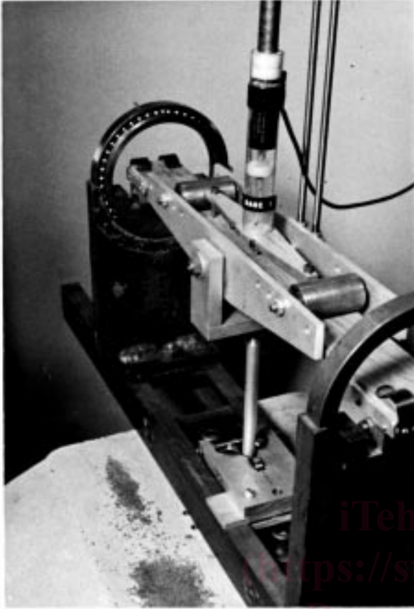
FIG. 3 Apparatus for Two-Point Loading and Measurement of Deflection (Method B)
