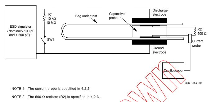
NOTE 3 Switch SW1 is closed 10 ms to 100 ms after the pulse delivery period to ensure that the discharge electrode is not left in a charged state. The switch should be open at least 10 ms prior to the delivery of the next pulse. R1 and SW1 are part of the ESD simulator's internal circuitry.
