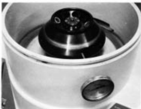
FIG. 1 Installation of Dial Thermometer (Sorvall Centrifuge)
