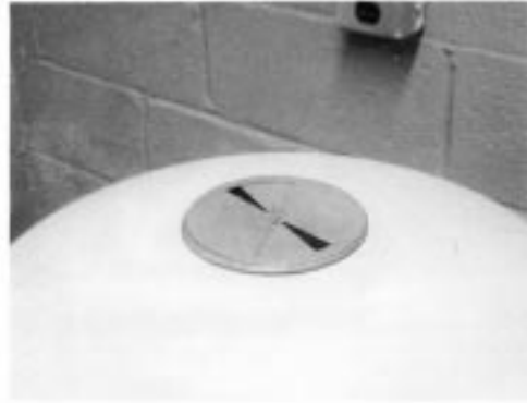
FIG. 2 Choking Air Inlet of Chamber (Sorvall Centrifuge)
