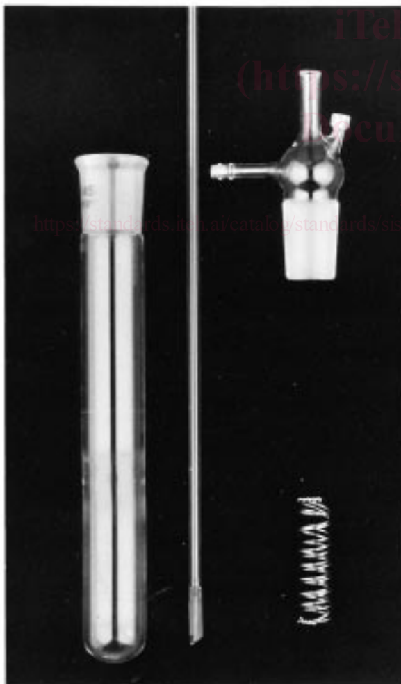
FIG. 2 Test Cell, Including Oxidation Cell, Gas Inlet Tube, Basic Head, and Finished Catalyst Coil
