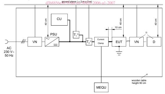
NOTE 1 The terminations  $T_1$  and  $T_2$  have to be used alternatively.  $T_1$  is used for minimum HBES configuration test.  $T_2$  is used for EUT test. The output either of  $T_1$  or  $T_2$  has to be terminated with 50  $\Omega$ /m to ground.
