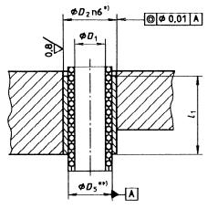
\*) Intended to fit in a hole having a tolerance H7.
