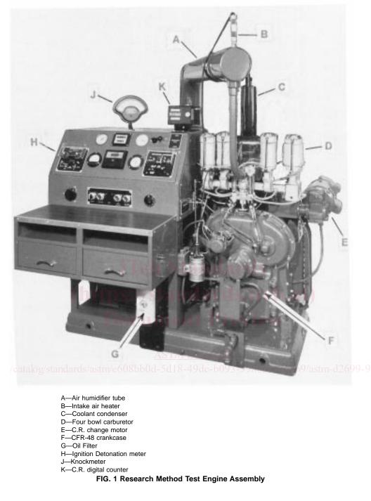
combustion knock as well as conventional thermometry, gages, and general purpose meters.
