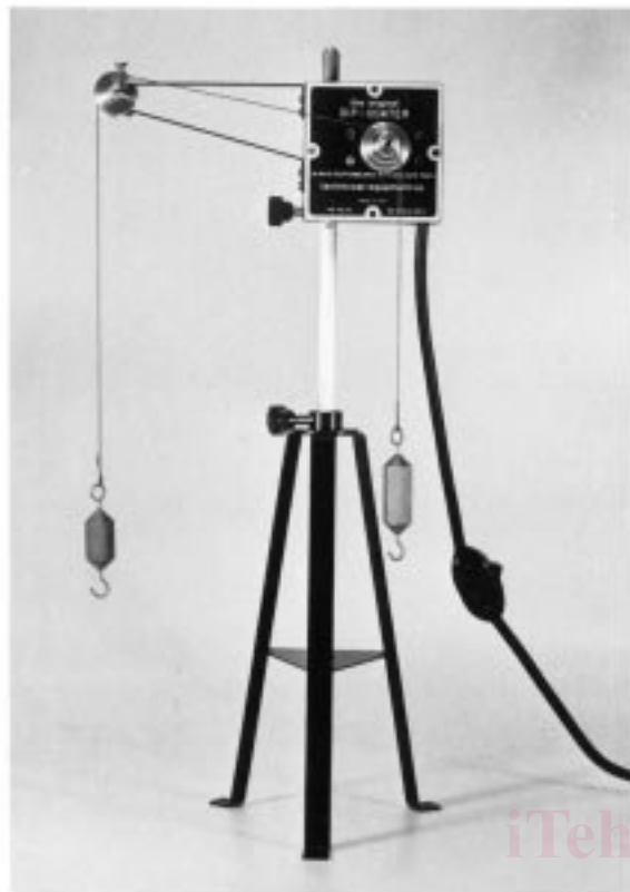
(a) Dip-Coater With Motor-Driven Step-Cone Pulley
