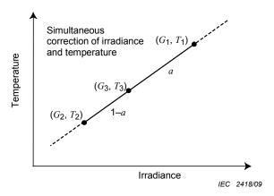
The solid line and broken line show the range of  $G_3$  and  $T_3$  which are calculable by the interpolation and extrapolation, respectively.
