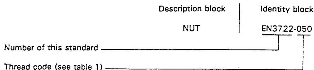
NOTE : If necessary, the code 19005 shall be placed between the description block and the identity block.
