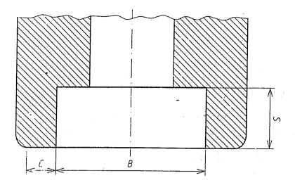
Figure 1 - Socket welding end detail
