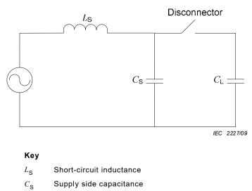
C<sub>1</sub> Load side capacitance
