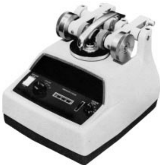
FIG. 1 Rotary Platform Double Head Abraser
