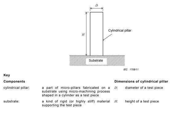
Figure 1 – Shape of cylindrical pillar (See Table 1 for symbols)
