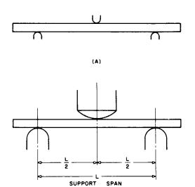
Note—(a) Minimum radius = 3.2 mm ( $\frac{1}{8}$  in.). (b) Maximum radius supports 1.6 times specimen depth; maximum radius loading nose = 4 times specimen depth.
