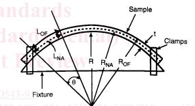
$\begin{array}{ll} R = \mbox{radius of jig} \\ R_{NA} = \mbox{radius of neutral axis} \\ R_{OF} = \mbox{radius of outer fiber} \\ t = \mbox{thickness of specimen} \end{array} \qquad \begin{array}{ll} \theta = \mbox{arbitrary angle} \\ L_{OF} = \mbox{length of outer fiber} \\ L_{NA} = \mbox{length of neutral axi} \end{array}$
