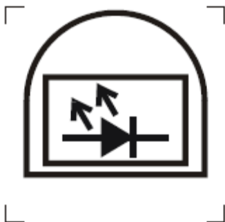
Figure 1 – Symbol for built-in LED modules
