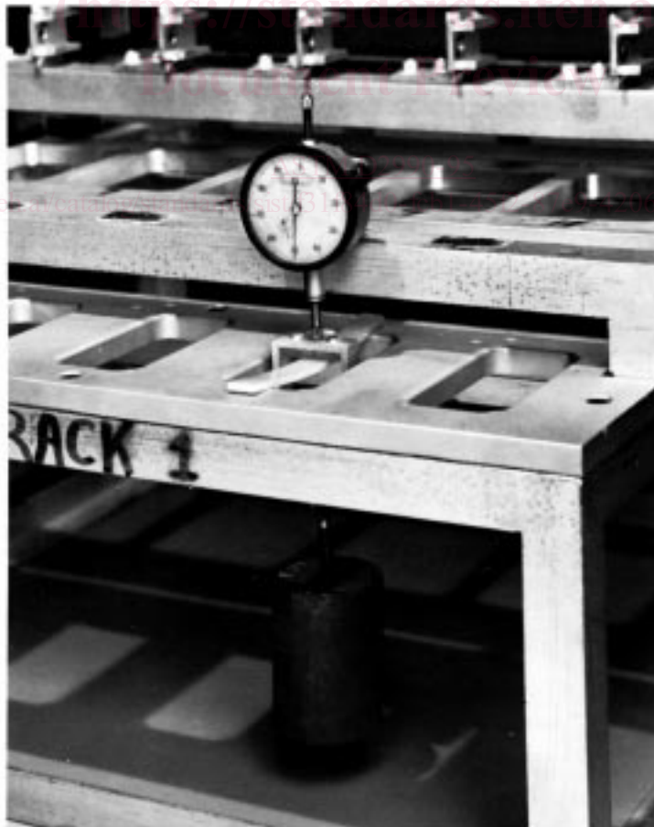
FIG. 2 Flexural Creep Test Apparatus
