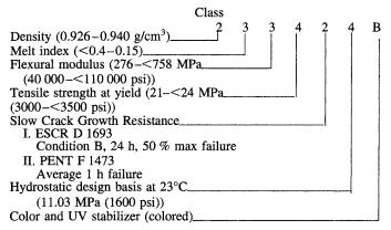
4.2 Materials used in polyethylene plastic pipe and fittings shall use a cell-type format for the identification, close characterization, and specification of material properties. The information from the format is to be used alone or in combination.
