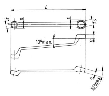
1) Overall dimensions of heads in accordance with ISO 3318, with the exception of the width across flats 20 mm, 23 mm, 25 mm and  $^{\circ}$
