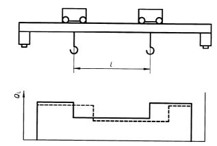
a) A minimum distance *l* between two crabs is required in order to use the full rated capacity of the crabs. With a shorter distance the rated capacity is reduced (mainly in order to reduce bridge weight and keep wheel loads within allowable limits).
